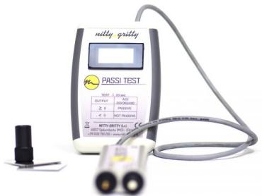
**Passi Test** is a tool designed for those who need to know exactly the real quality of the stainless steel. It consists of a “probe pen” – which will be put on the superface to be tested – containing the electrochemical system and a reading external unity. **Passi Test** measures the open-circuit potential and the nobility of a metal (and consequently its resistance to corrosion).
