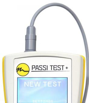
**Passi Test Plus** is a tool designed to assess the real quality of stainless steel. It consists of a “probe pen”, which contains the electrochemical solution, and an external storage unit. By pressing the probe pen on the surface, Passi Test Plus measures and stores data on the open-circuit potential and nobility of a metal, thus measuring its corrosion resistance.
